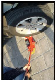
Raise the vehicle enough to remove the axle stands, then slowly lower the lifting jack.
