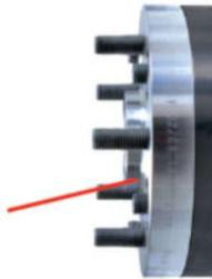
System 3 - 14xxx You must consider that the original vehicle studs can protrude the mounting surface of the new spacer (15, 20, 25 and 30mm). If the wheel has no reiler pockets then the vehicle studs will need to be shortened to allow the wheel to sit flat to the mounting face of the spacer. This will always apply to System 3 15mm.
