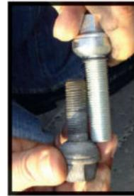
*Check if the length and type of sealing of the new and longer bolts are correct. (Have a look overleaf at the bolts advice. The new fixings need to be as long as the originals plus the thickness of the spacer.*
