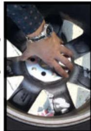
*Check that the spacer is completely in contact with the mounting surface of the wheel.*
