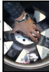
Check that the spacer is completely in contact with the mounting surface of the wheel.
