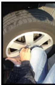
Locate the wheel, fix with the new nuts/bolts and tighten by hand.
