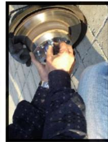
Mount the wheel spacer on the axle using the nuts/bolts which were included in the delivery. Tighten the nuts/bolts by hand.
