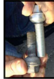
Check if the length and type of sealing of the new and longer bolts are correct. (Have a look overleaf at the bolts advice. The new fixings need to be as long as the originals plus the thickness of the spacer.
