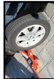
Lift the vehicle until the tire is off the ground, then place an axle stand under the vehicle.
